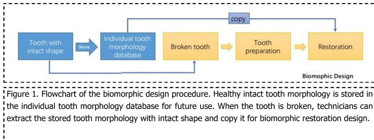
Figure 1. Flowchart of the biomorphic design procedure. Healthy intact tooth morphology is stored in the individual tooth morphology database for future use. When the tooth is broken, technicians can extract the stored tooth morphology with intact shape and copy it for biomorphic restoration design.
